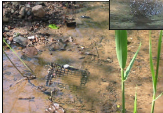
Fabric pads, contained in metal cages, were placed in streams to absorb optical brighteners.
