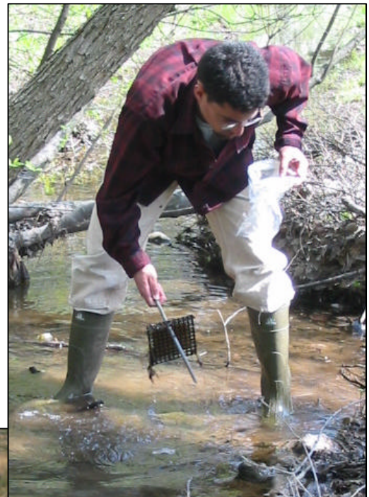
Fabric pads, contained in metal cages, were placed in streams to absorb optical brighteners.
